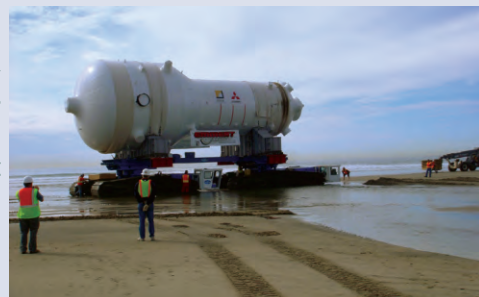
Transport of a replacement steam generator through Camp Pendleton, including crossing of the Santa Margarita River.
