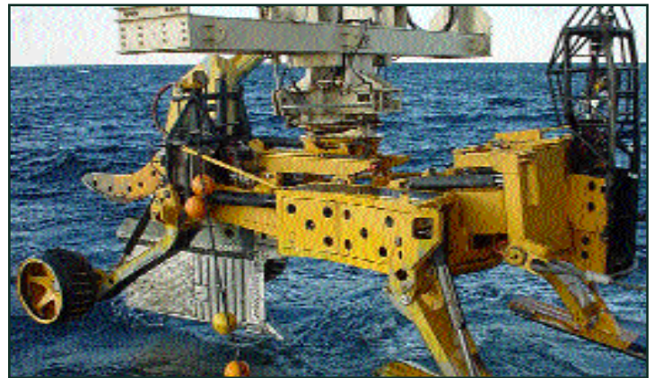
Plow used for cable laying operations
